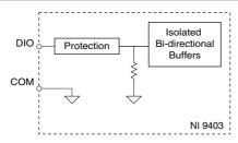
The DIO channels have Schmitt trigger inputs and are compatible with 5 V/TTL logic devices. Each input channel has hysteresis for improved performance with noisy and non-monotonic input signals. Each channel also has a pull-down resistor.
