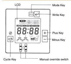
**Note:** This figure shows the LCD section with all display items being displayed on the screen.
