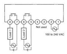
Note: To each load, connect the power supply for load.
