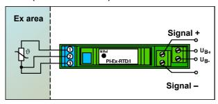
Figure 5 3-wire resistance thermometer
