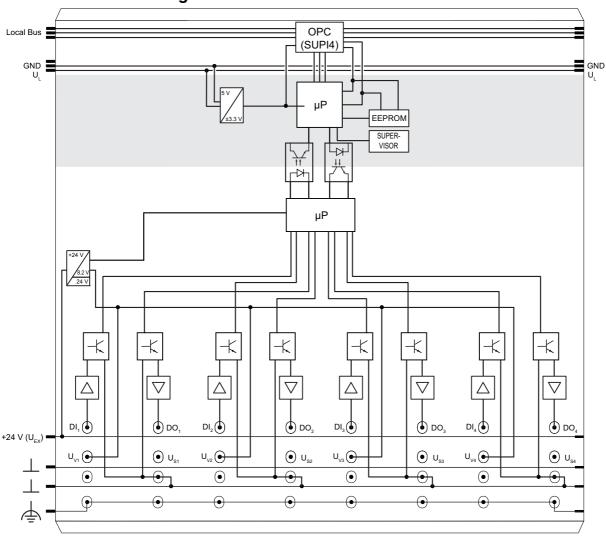
Figure 1 Internal wiring of the terminal points
