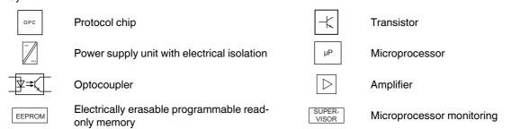
Other symbols used are explained in the IB IL SYS PRO UM E user manual or in the Inline system manual for your bus system.
