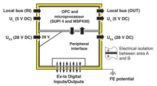
Figure 2 Electrical isolation of the individual function areas
