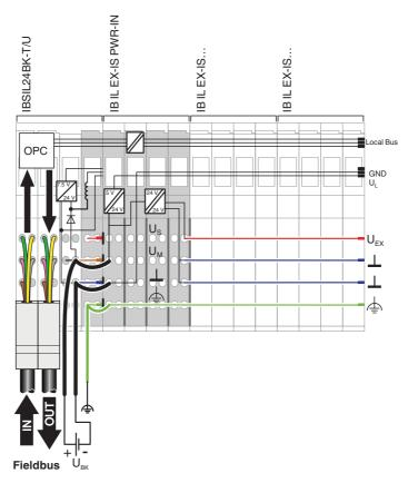
Figure 4 Intrinsically safe Inline terminals power supply
