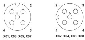
Figure 6 Pin assignment of the inputs and outputs, A-coded
