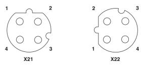
Figure 3 Ethernet pin assignment, D-coded
