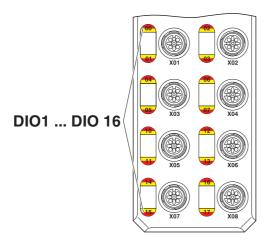
Figure 10 Input and output indicators
