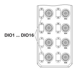
Figure 5 Input and output connections
