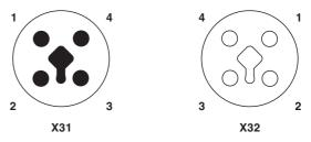
Figure 4 Pin assignment of the power supply, T-coded
